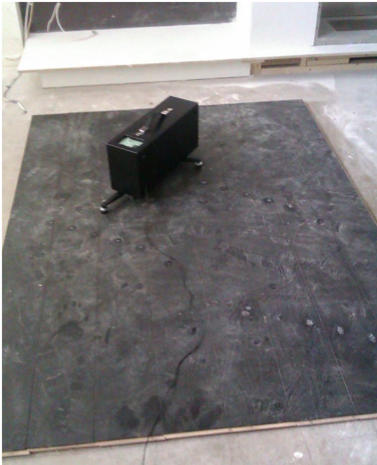
Figure 1: Tapping machine in-situ
